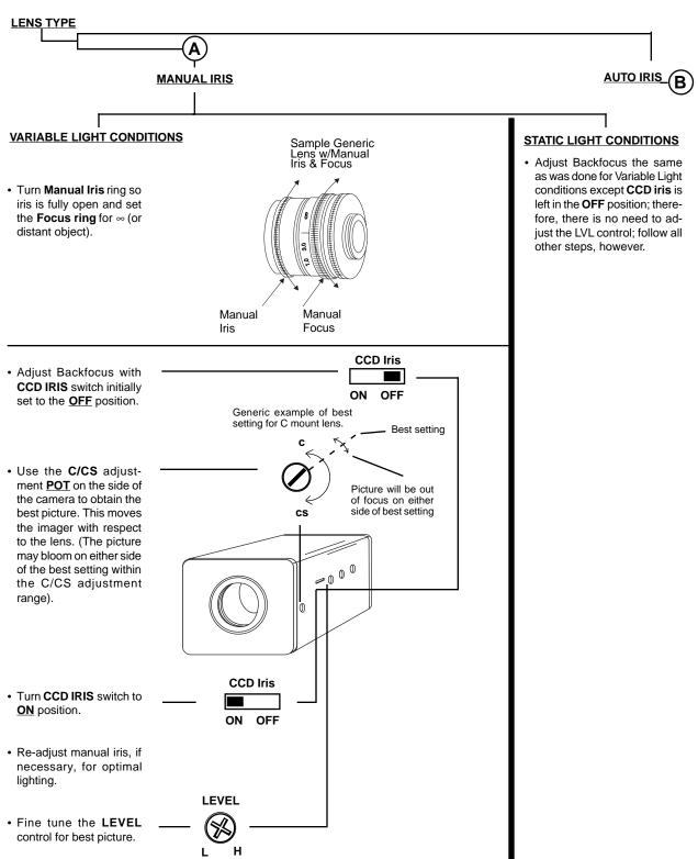
The purpose of backfocusing is to make the adjustments necessary for the picture to remain in focus throughout the camera's zoom range, which is the case for instance, in motorized zoom, auto iris configurations. Manual Iris lens/camera combinations also need to be backfocused. Follow the general instructions listed below to adjust backfocus appropriate to your camera/lens combination.
